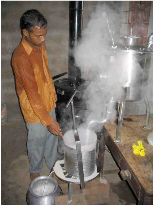
Soy milk Production showing Cooker (on table) and Press below
